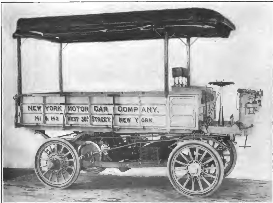
NEW ATLAS TWO-TON TRUCK, FITTED WITH 24-HORSEPOWER WATER-COOLED MOTOR, BUILT BY HARRY A. KNOX AT SPRINGFIELD, MASS., FOR HIS NEW YORK AGENCY.
